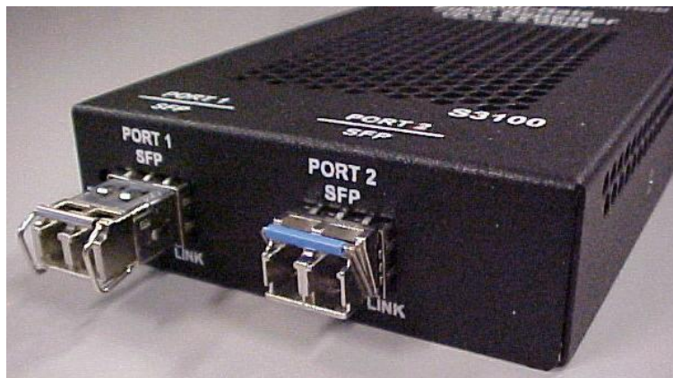
Figure 3: Port Locations and SFP Installation
