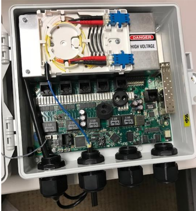
Fig. 5: Fiber Tray with Fiber (Installed)
