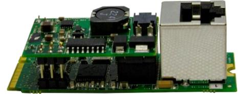
The SESP-2P-24V-CP is a Passive PoE Port Module to provide 24VDC power over a 10/100/1000Base-T port. Alternatively, it could also be used to activate a second 100/1000Base-X combo port (no passive PoE is provided over fiber). **Note:** Refer to the switch, module, and attached device documentation for important related information.
