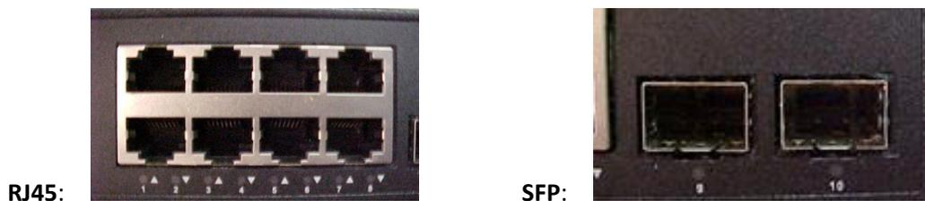
Figure 10: RJ-45 and SFP Ports
