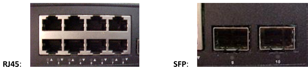
Figure 10: RJ-45 and SFP Ports
