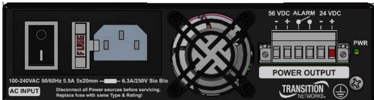
PS-DC-DUAL-5624T Hardened 345 Watt Isolated Power Supply with 56VDC and 24VDC Dual Output
